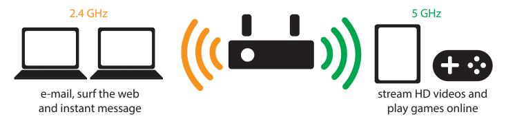
For home networks, those devices that have the capacity to handle the most data – gaming systems, desktop or laptop computers or your Internet –enabled TV systems, should be connected to your 5.0 for the fastest speeds. Think line of sight – if you can see the router or you have an open window, thin wall or a cubicle wall in between, 5.0 would be the best bet. Everything else? 2.4.
